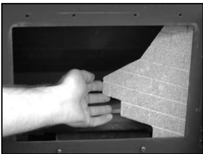
Fig. 3b Fitting the R/H side lining
