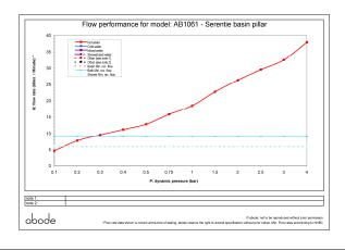
• Min / Max water pressure: 0.20 / 5 bar • Part G mixed flow rate at 3 bar (I/m): 32.5
