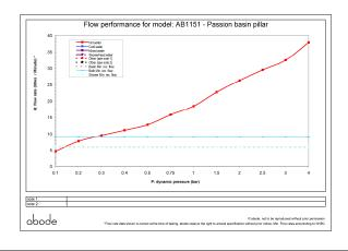
• Min / Max water pressure: 0.20 / 5 bar • Part G mixed flow rate at 3 bar (I/m): 32.5
