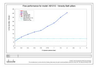
• Min / Max water pressure: 0.20 / 5 bar • Part G mixed flow rate at 3 bar (I/m): >81.4
