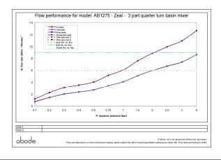
• Min / Max water pressure: 1.00 / 5 bar • Part G mixed flow rate at 3 bar (I/m): 10.95
