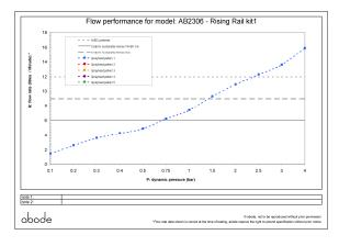
Min / Max water pressure: 0.75 / 5 bar
