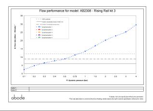
• Min / Max water pressure: 0.30 / 5 bar • Part G mixed flow rate at 3 bar (I/m): 25.3
