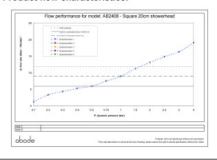
• Min / Max water pressure: 0.40 / 5 bar • Part G mixed flow rate at 3 bar (I/m): 16.4
