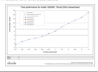
• Min / Max water pressure: 0.30 / 5 bar • Part G mixed flow rate at 3 bar (I/m): 14.64
