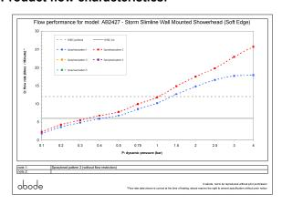
Min / Max water pressure: 0.80 / 5 bar
