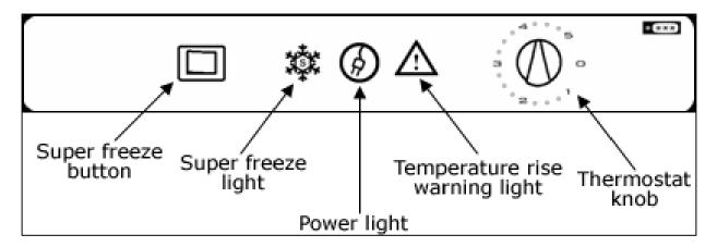
You switch on your appliance by connecting it to your mains supply and setting the thermostat. The thermostat is located on the control panel, at the top of the freezer.
