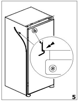
**5)** Cut the sealing strip so that is the same height as the height of the aperture.
