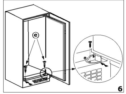
Slide the appliance over to the far left of the aperture, unless you have reversed the door. In which case you should slide the appliance over to the far right of the aperture.
