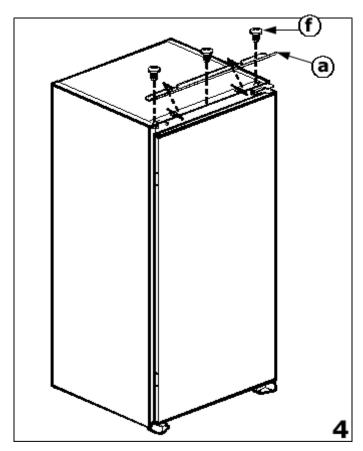
4) Insert the top fixing bar
