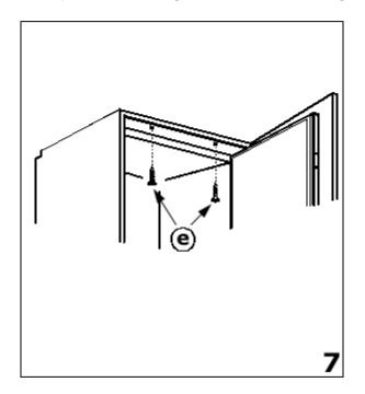
**7)** Screw the top fixing bar to the underneath of the kitchen unit using the  $\emptyset 4 \ge 17$  fixing screws (e).
