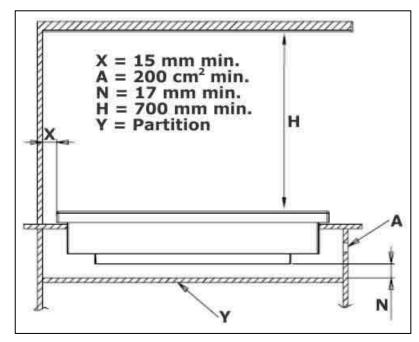
o **IMPORTANT:** Underneath the appliance there must be a partition made of insulating material (e.g. wood). There must be
