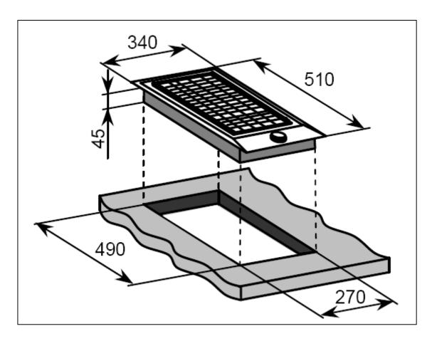
o Cut a hole in the worktop that corresponds with the drawing shown above.
