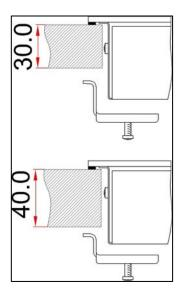
Use the fixing bracket that is appropriate for your thickness of worktop.
