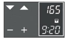
To deactivate the safety lock, press and hold the power button for 3 seconds again. The safety lock icon on the LCD display will show an open padlock to indicate that the safety lock has been deactivated and the controls can now be operated.
