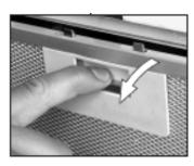
**1)** Remove the grease filters (as previously described).
