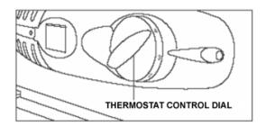
You switch on your appliance by connecting it to your mains supply and setting the thermostat. The thermostat control knob is located on the right hand side of the fridge.
