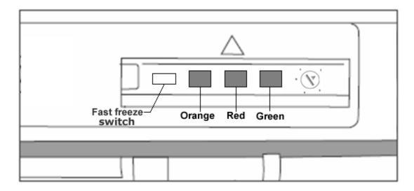
Press the fast freeze switch and the freezer will start to run continuously at its maximum setting.
