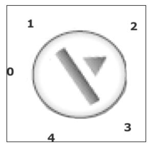
You switch on your appliance by connecting it to your mains supply and setting the thermostat. The thermostat control knob is located at the top of the appliance.
