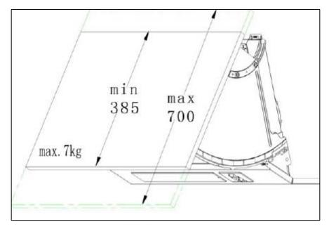
The décor door should be no less than 16 mm thick, 385 – 700 mm high and weigh no more than 7 kg.
