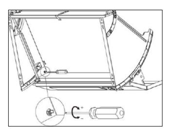
The two screws on both sides of the cooker hood can be adjusted to alter the sliding of the door, according to its weight.
