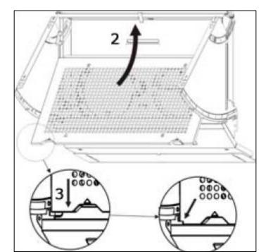
o Ensure the filter unclips from the hood, as shown in the diagram on the previous page, before you pull it away. This will allow you access to the motor where the carbon filter should be fitted.
