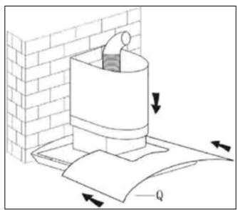
o Carefully place the glass section (Q) on the upper surface of the cooker hood and then slide it back towards the wall.
