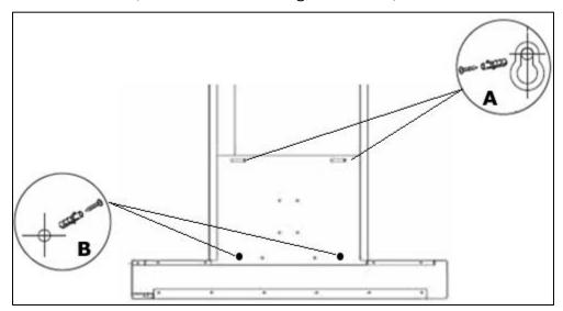
**2a)** The support screw holes are indicated by figure  ${\bf A}$  in this drawing and the anchoring screw holes are indicated by figure  ${\bf B}$ .
