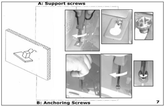
7) Fully tighten the support screws (A) and then screw the anchoring screws (B) through the relevant holes in the cooker hood. Tighten the anchoring screws fully into the wall.
