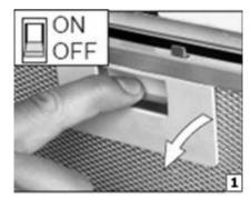
1) Remove the grease filter.
