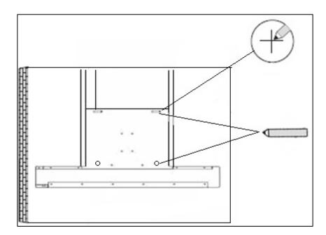
**2)** Position the hood against the wall that you are intending to install it on and mark the position of the support holes that are to be drilled (as shown in the figure below).
