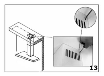
**13)** Lift chimney section  $\mathbf{D}$  up to the ceiling and secure it to the fixing bracket using the screws provided.
