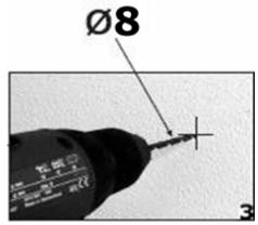
**3)** Using a drill bit with a 8 mm diameter, make holes in the wall on the positions that you have marked in step 2.
