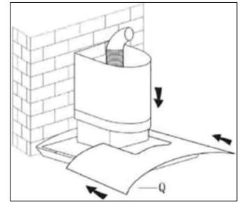
• Carefully place the glass section **(Q)** on the upper surface of the cooker hood and then slide it back towards the wall.
