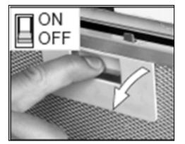
First remove the grease filter by pulling down on the handle and pulling them away from the cooker hood.
