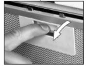
**1)** Remove the metal grease filters.
