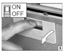
1) Remove the grease filters.
