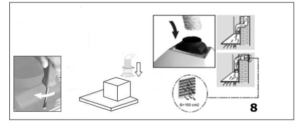
**8)** Connect the coupling to the top of the cooker hood, and then connect a 125 mm ducting hose to the coupling (please note that the ducting hose is not supplied with the appliance).
