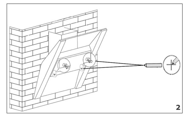
**2)** Position the hood against the wall that you are intending to install it on and mark the position of the screw holes that are to be drilled (as shown in the figure below).
