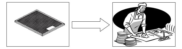
Soak the grease filters in hot water and washing up liquid for at least 3 minutes. Then use a soft brush to loosen any grease deposits that have formed.
