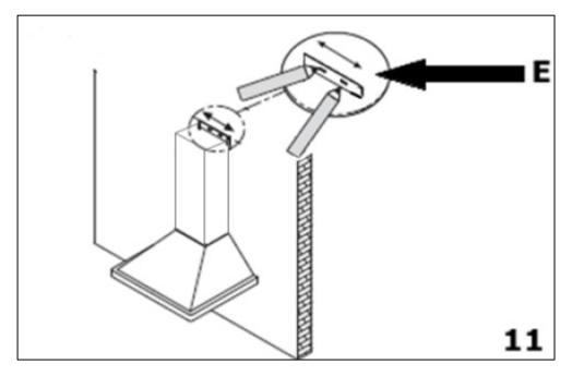
**11)** Take the flat bracket **(E)** and place it between the two pencil marks that you made in step 9
