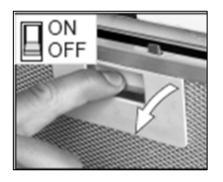
First open the cover screen and remove the grease filters (as previously described).
