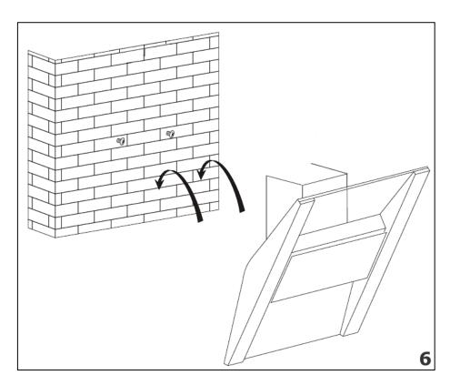
6) Hang the hood onto the support screws.
