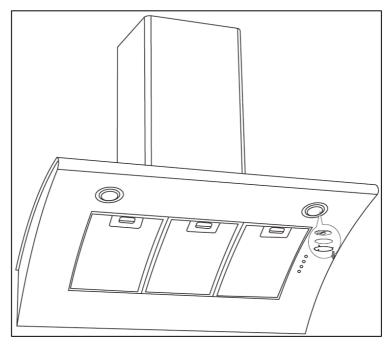
Prior to touching the light bulbs ensure that they have cooled down.  Find the bulb that requires replacement, you will find it located in the light fixture which is inside the exposed section of the canopy.
