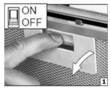
1) Remove the grease filters.
