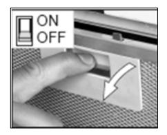
Refit the grease filters.
