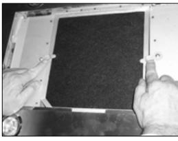
4) After inserting the front edge of the carbon filter into the slot on the cooker hood. Lower the back edge of the carbon filter, until it clicks into place at the rear of the rectangular hole. Raise the two fixing bars, until they are horizontal over the carbon filter.
