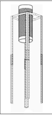
**4)** If your cooker hood is going to be used in extraction mode, then you should connect the ducting hose to the ceiling adaptor at this point.
