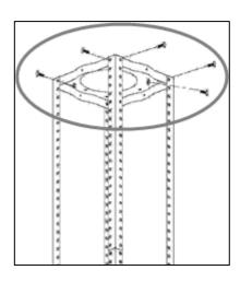
**2)** Fix the angle bars to the hanging plate, using the  $8 \times M4$  nuts and bolts with metal washers.
