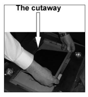
3) Insert the carbon filter in the rectangular hole, fitting it over the motor.
