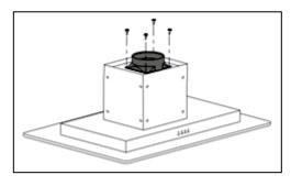
**6)** If you are going to be using the hood in extraction mode, you should fit the spigot for the duct hose onto the main body of the cooker hood, using the 4 x M4 bolts,
