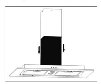
Remove the hanging hook and then slide the lower chimney section downwards, until it rests against the main body of the cooker hood.
