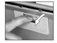
1) Remove the metal grease filters.
