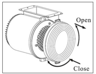
2) Press the carbon filter against one end of the motor, the fixing point is in the centre of the carbon filter.
