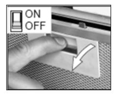
Refit the grease filters.
