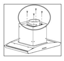
**5)** If you are going to be using the hood in extraction mode, you should fit the spigot for the duct hose onto the main body of the cooker hood, using the 4 x M4 bolts,
