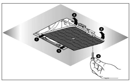
1) Locate the SCS14 carbon filter into the slots on the cooker hood, below the motor.
