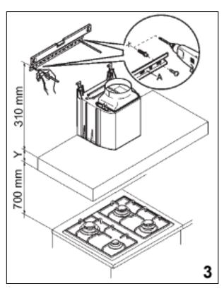
mm from the hob top that will be underneath the cooker hood. Then measure out a further 310 mm above the height of measurement Y (Y being the thickness of the canopy section of the cooker hood).
