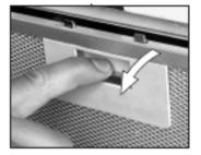
**1)** Open the cover screen and remove the metal grease filters.
