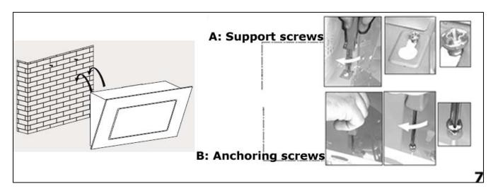
7) Fully tighten the support screws (A) and then screw the anchoring screws (B) through the relevant holes in the cooker hood. Fully tighten the anchoring screws into the wall.
