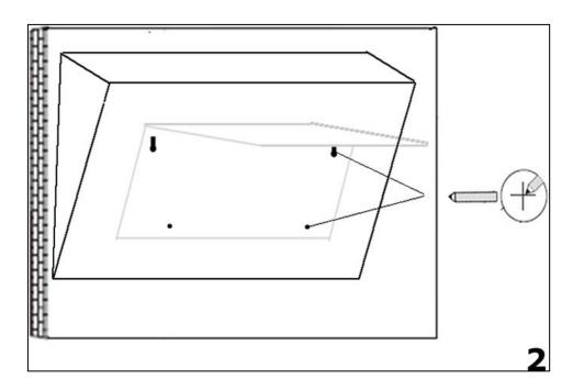
**2)** Position the hood against the wall that you are intending to install it on and mark the position of the screw holes that are to be drilled (as shown in the figure below).
