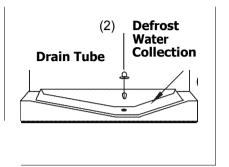
check to ensure that no food particles have blocked the drain tube. The drain tube can be cleared by pushing the special plastic plunger provided down the drain tube (2). If the frost layer reaches about 1 /4"(7 mm), reduce the setting (i.e. from 4 to 1) to restart automatic defrosting.
