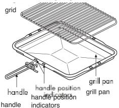
Place the handle over the edge of the grill pan, at the narrow side edges. Slide the handle to the centre, and locate between the handle position
