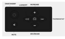
**NOTE:** The manual keypad on the appliance will provide you with complete functional control of the unit. It is intended however that this keypad is used only if you lose the remote handset or the handset batteries have failed. Please use the remote handset to carry out all functions
