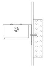
**Note.** Depending on the nature of the cabinet it may be necessary to position a batten behind the panel to make a secure fixing. Remember the weight of the housing will increase when filled with water.
