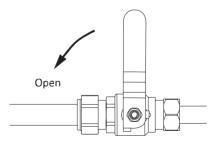
7. Turn the water supply 'on' and check the system carefully for leaks. Leave the filter tap in the 'on' position and allow the water to run for a minimum of 10 minutes to flush the system. Check the flow rate. We recommend no more than 30 seconds a litre for optimum performance. If the flow is too fast it can be regulated by adjusting the stop valve.
