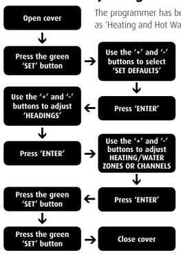
The programmer has been preset to display the channel heading as 'Heating and Hot Water', should you require either the 'Zone'
