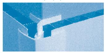
To form an external corner fix the mounting strip to the wall using wall plugs and flat head screws. Finish corner by clipping the front face into place.
