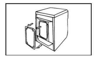
o Remove the back plate from the rear of the appliance.
