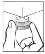
✓ Adjust the feet to level off the washing machine.
