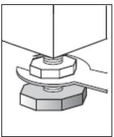
✓ Once levelled correctly, you should tighten the lock nut back up on each of the washing machine feet using a spanner.
