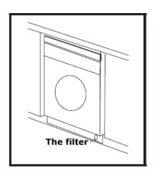
Locate the drain pump filter in the bottom right hand corner of the appliance.
