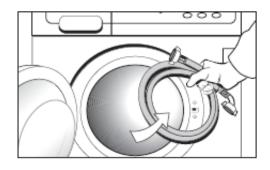
The water inlet hoses will be inside the drum of your washing machine, when you receive the appliance.
