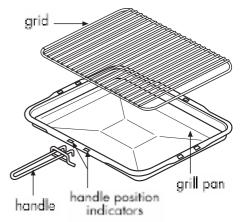
Place the handle over the edge of the grill pan, at the narrow side edges. Slide the handle to the centre, and locate between the handle position indicators.
