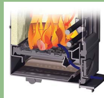
Grate and PADS set for wood burning, providing an over draught to the fuel bed.
